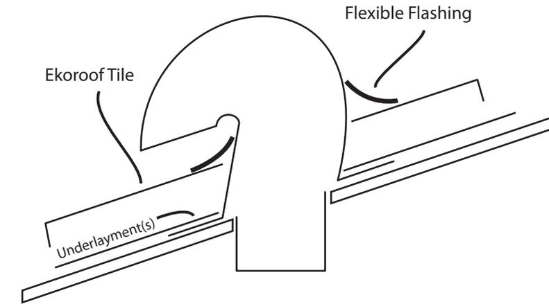
Recommended flexible flashing brand is DEKS® brand KwikFlash® with aluminum mesh
