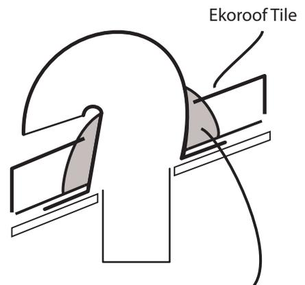
Fully seal gooseneck to Ekorooftile using Roofing Mortar color-matched to tile for aesthetics
