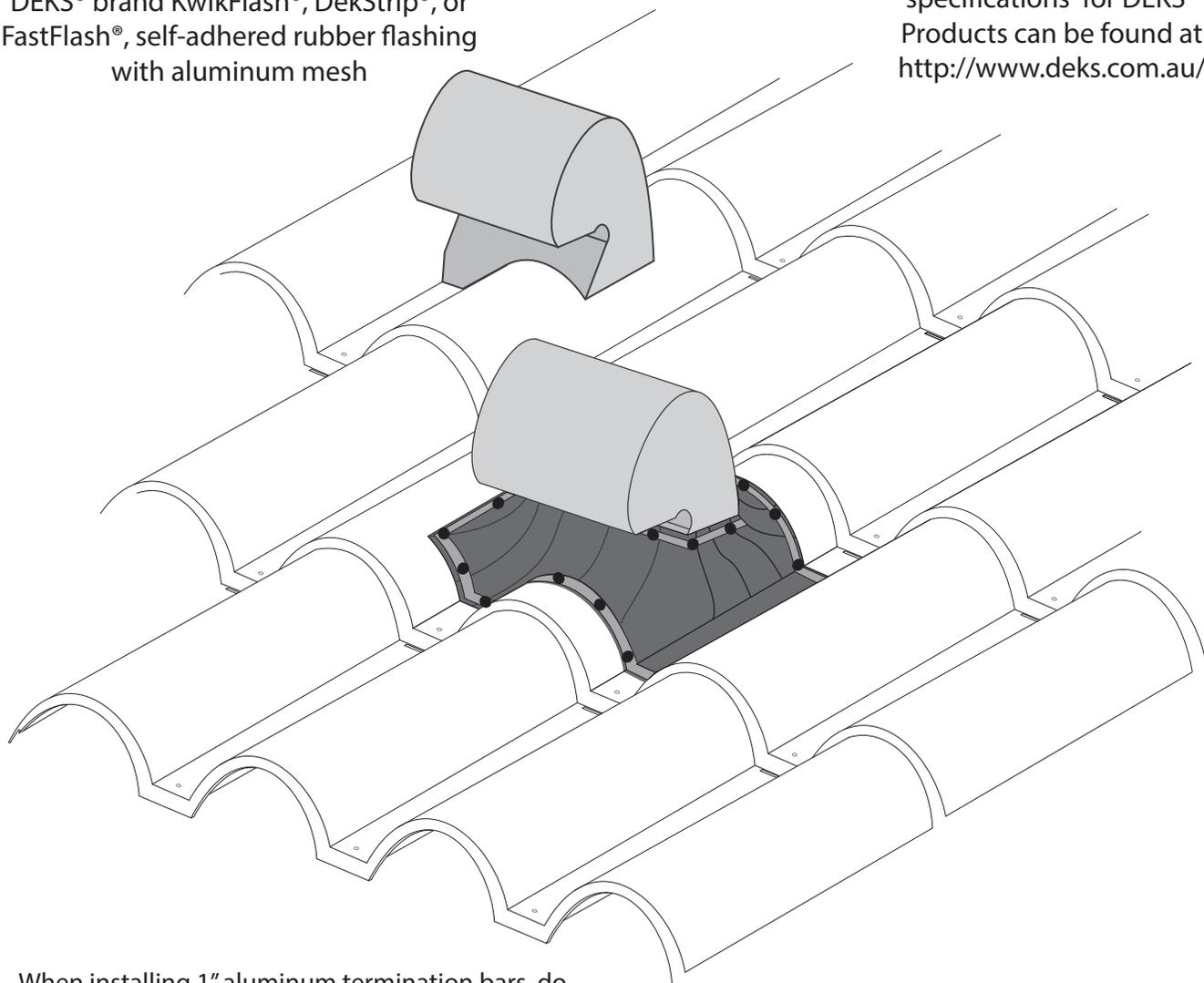
When installing 1" aluminum termination bars, do not penetrate underlayment(s) or sheathing. If penetrating deck cannot be avoided due to vent location, such as in a low point of tile, use 2" main Ekorooft fastener, color-matched for aesthetics.
